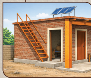
Stairs to rooftop enabling immediate personal safety during floods
